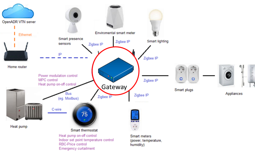
Figure 7. Example of HEMS serving as DR gateway, energy management system and controller.
